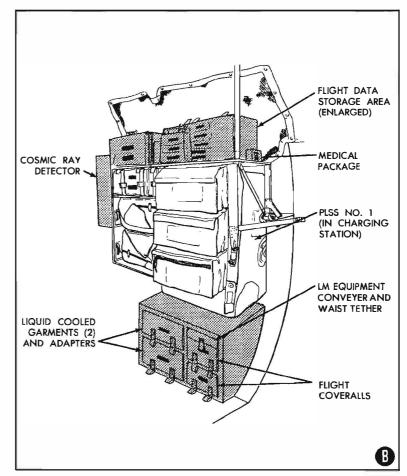
Figure 3-12.1. LM Crew Equipment Arrangement (Sheet 2 of 2)
