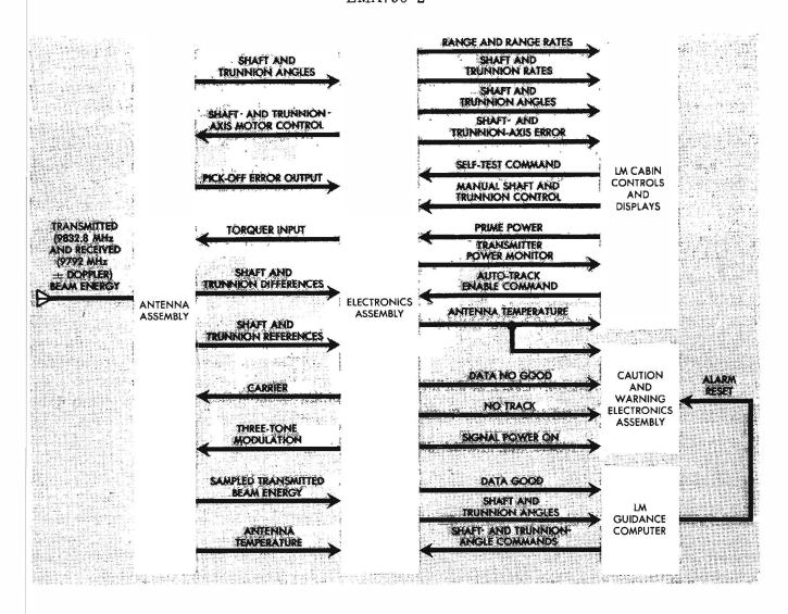
Figure 3-3.2. Rendezvous Radar-Signal Flow
