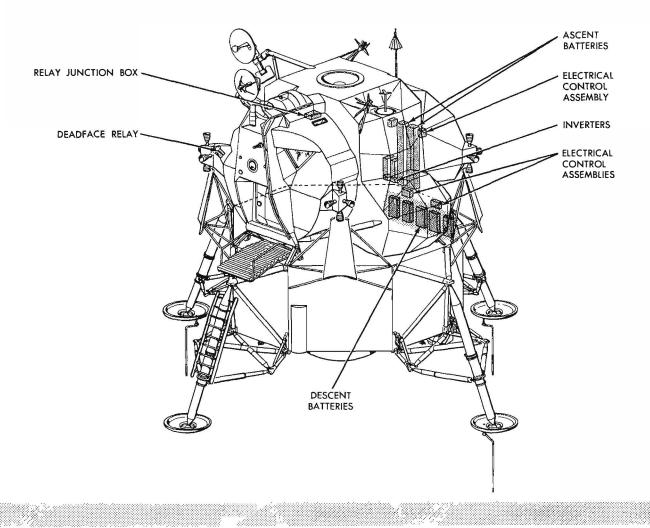
Figure 3-6.1. Electrical Power Subsystem - Major Equipment Location
