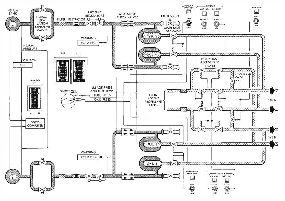
Figure 3-5.2. Helium Pressurization and Propellant Feed Sections - Flow Diagram
