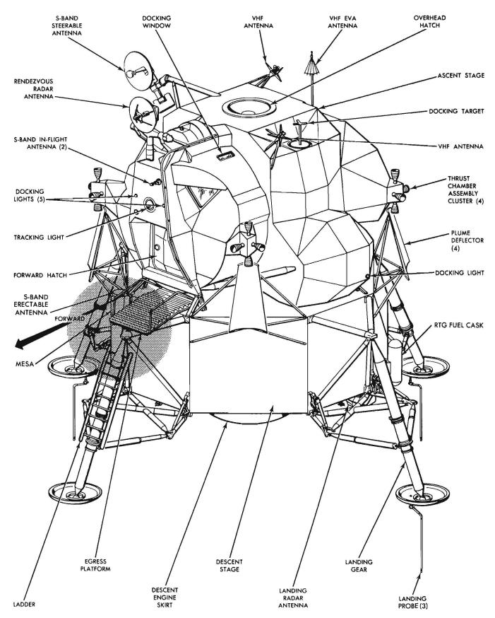
Figure 2-1. Vehicle Configuration
