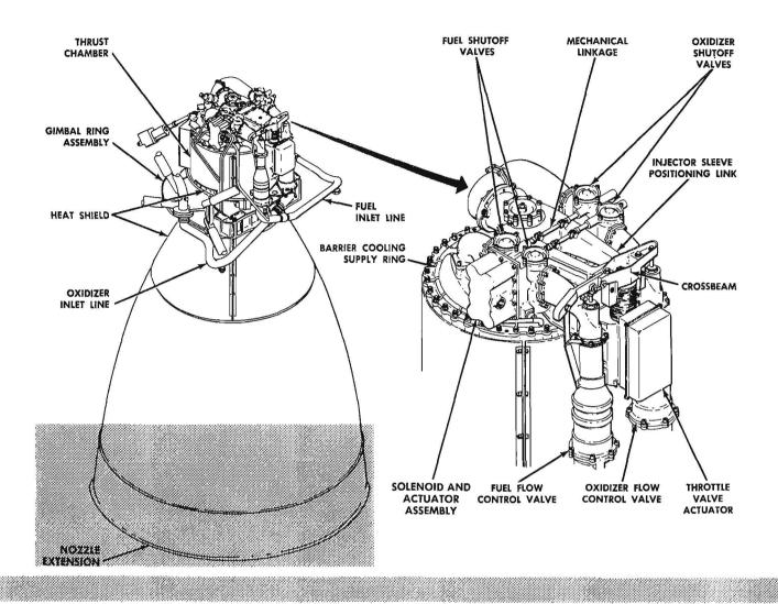
Figure 3-4.4. Descent Engine and Head End Assembly
