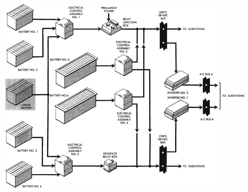
Figure 3-6.2. Electrical Power Subsystem - Flow Diagram
