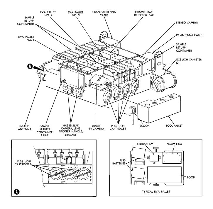
Figure 3-12.4. Modularized Equipment Stowage Assembly
