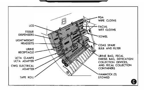
Figure 3-12.1. LM Crew Equipment Arrangement (Sheet 1 of 2)
