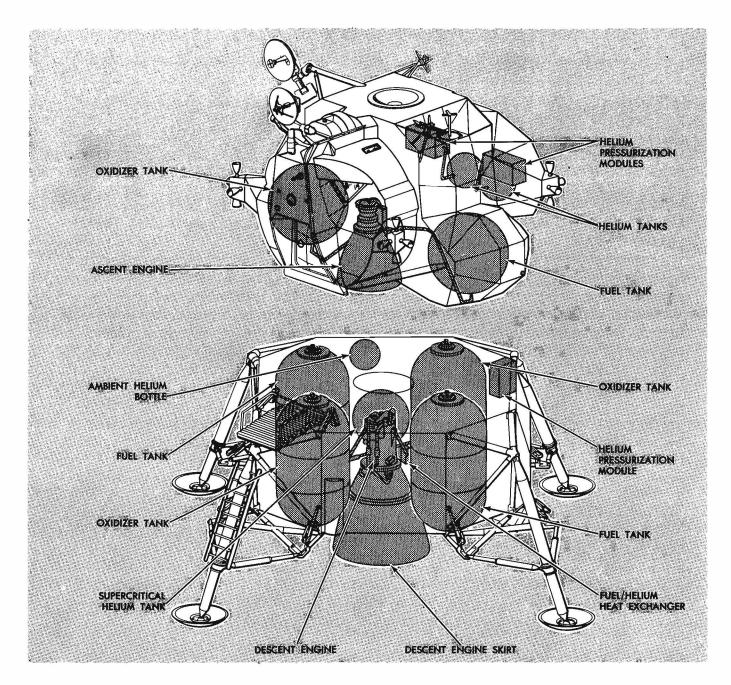
Figure 3-4.1. Main Propulsion Subsystem - Major Equipment Location
