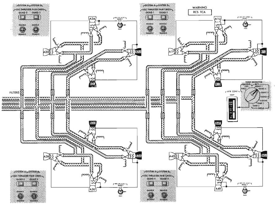
Figure 3-5.3. Propellant Lines and Thrusters - Flow Diagram
