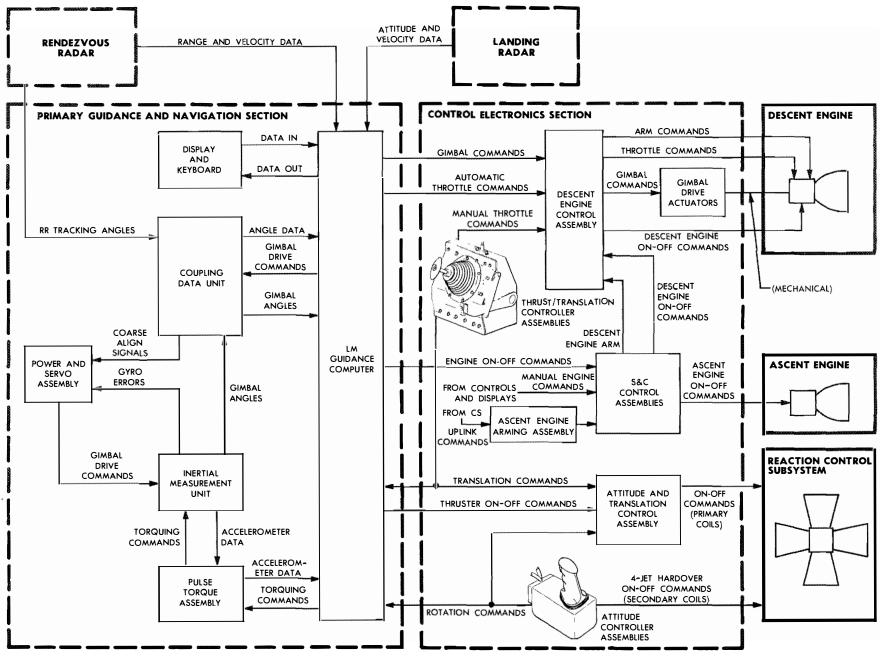
Figure 3-2.4. Primary Guidance Path - Simplified Block Diagram
