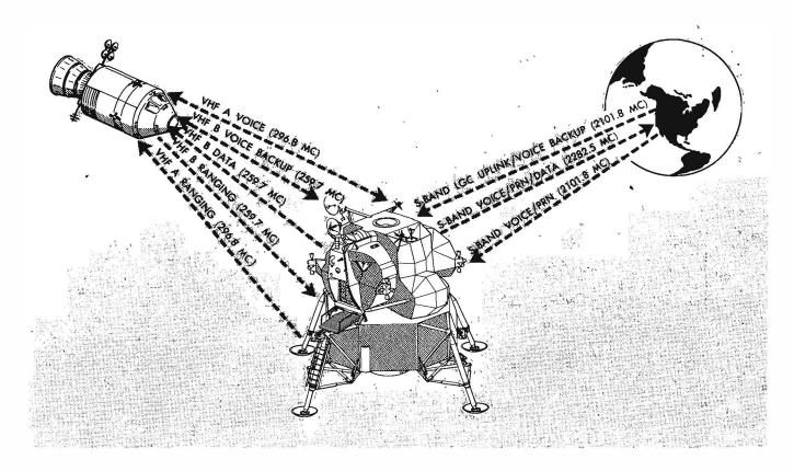
Figure 3-8.4. In-Flight Communications
