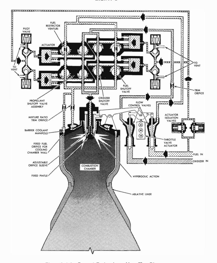
Figure 3-4.3. Descent Engine Assembly - Flow Diagram
