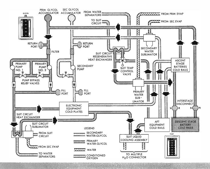
Figure 3-7.4. Heat Transport Section - Flow Diagram
