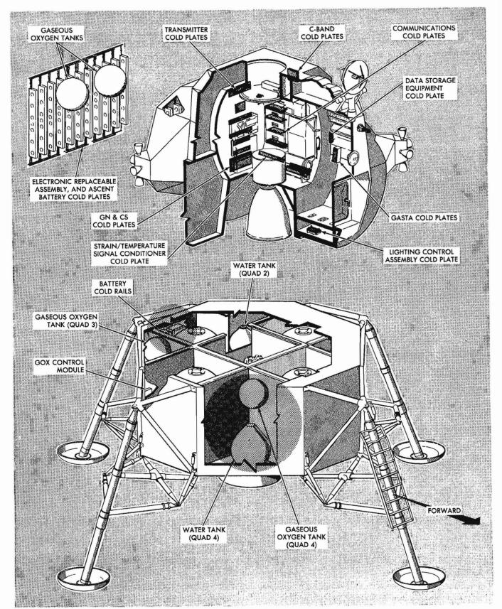
Figure 3-7.1. Environmental Control Subsystem - Component Location (Sheet 1 of 2)
