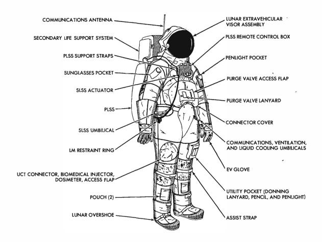
Figure 3-12.3. Integrated Thermal Micrometeoroid Garment
