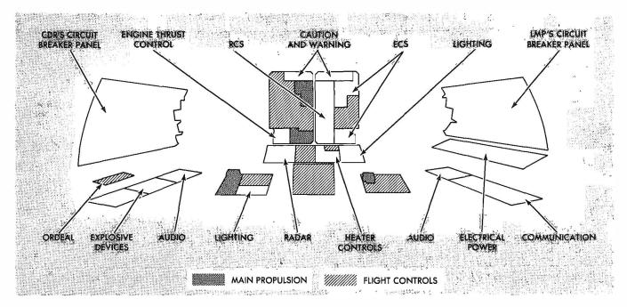
Figure 3-13.1. Controls and Displays - Subsystem Group
