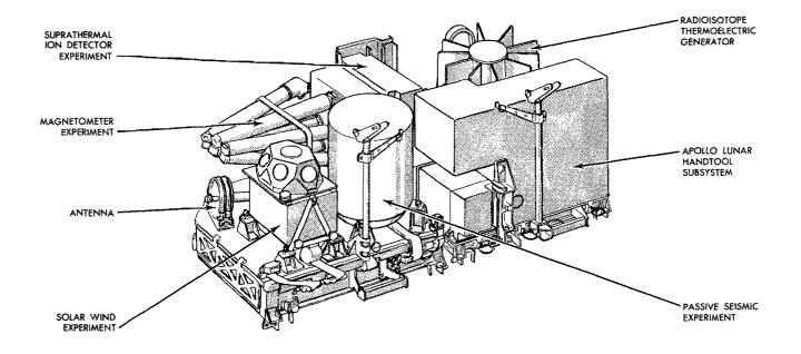
Figure 3-12.5. Apollo Lunar Surface Experiment Package
