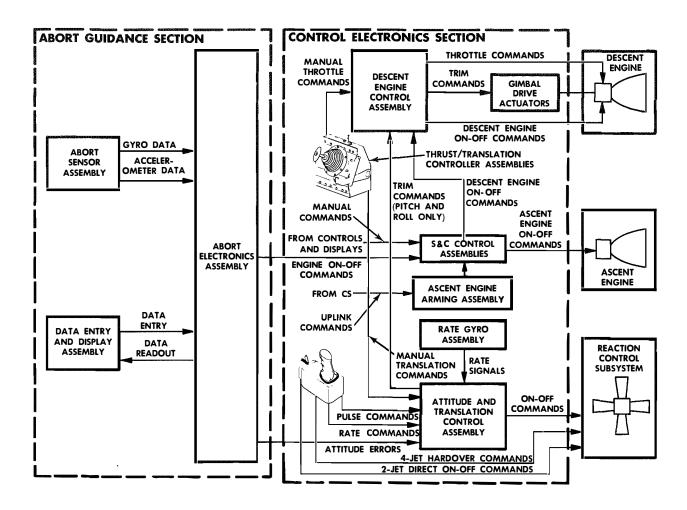
Figure 3-2.5. Abort Guidance Path - Simplified Block Diagram
