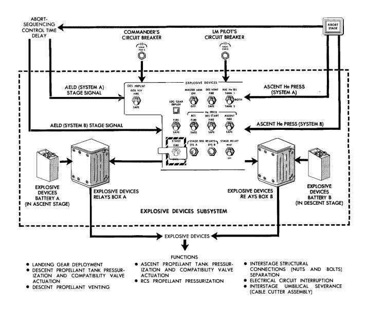
Figure 3-9.1. Explosive Devices Subsystem - Flow Diagram
