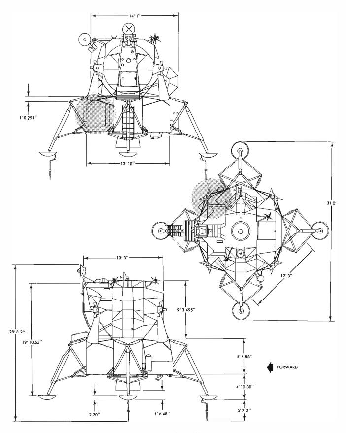
Figure 2-2. Vehicle Overall Dimensions
