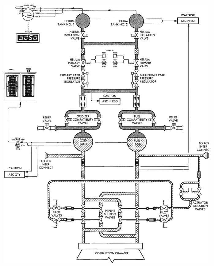
Figure 3-4.5. Ascent Propulsion Section - Flow Diagram
