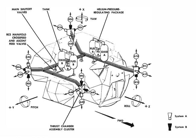
Figure 3-5.1. Reaction Control Subsystem - Major Equipment Location
