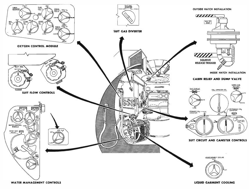
Figure 3-7.1. Environmental Control Subsystem - Component Location (Sheet 2 of 2)
