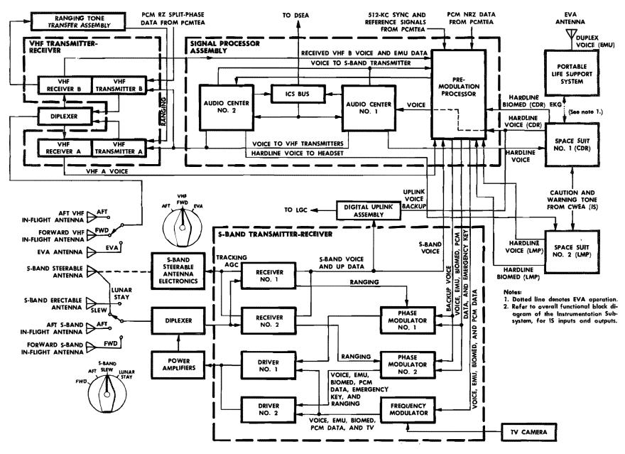
Figure 3-8.2. Communications Subsystem - Simplified Block Diagram
