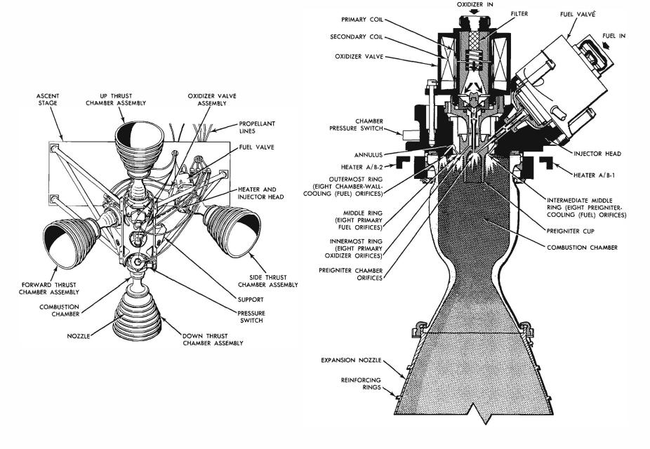
Figure 3-5.4. Thrust Chamber Assembly and Cluster
