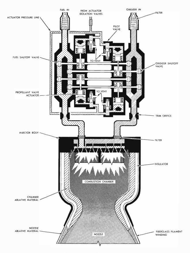
Figure 3-4.6. Ascent Engine Assembly - Flow Diagram
