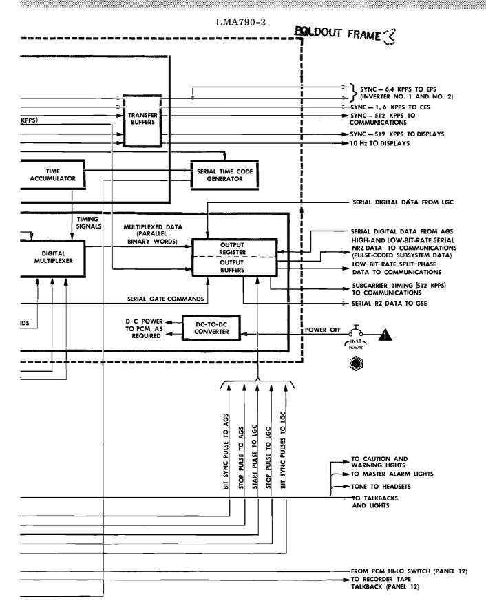
Figure 3-10.1. Instrumentation Subsystem - Block Diagram
