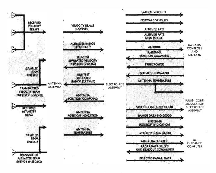
Figure 3-3.1. Landing Radar-Signal Flow
