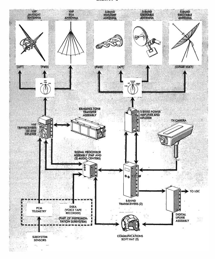
Figure 3-8.1. Communications Subsystem - Flow Diagram
