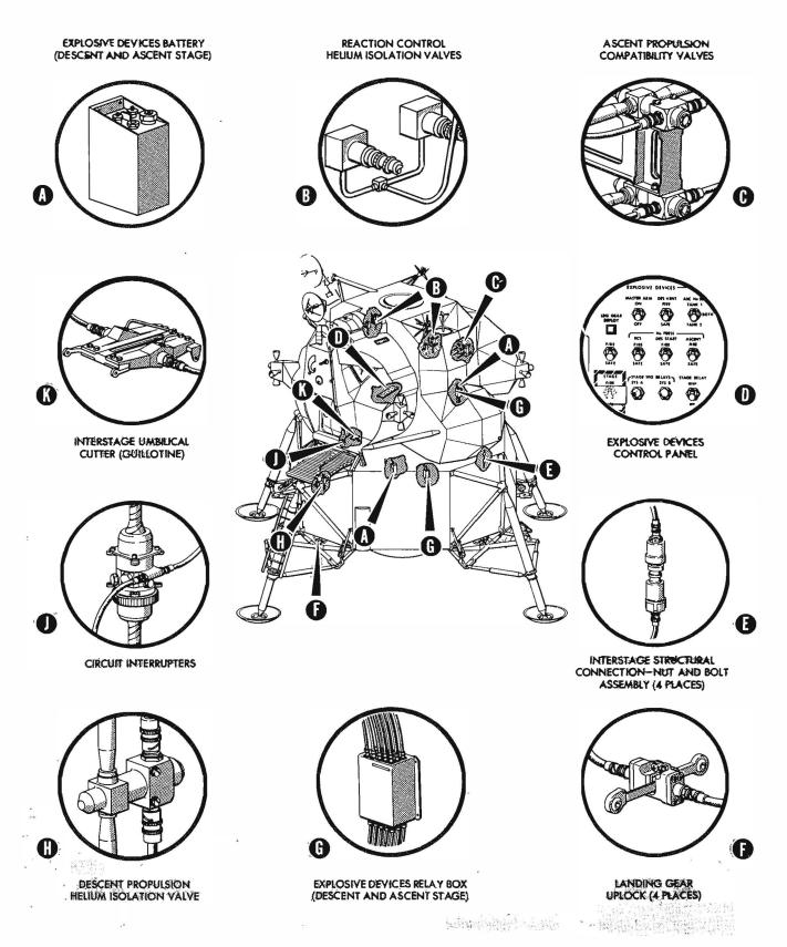
Figure 3-9.2. Explosive Devices Subsystem - Equipment Location
