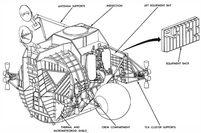
Figure 2-3. Ascent Stage Structure Configuration
