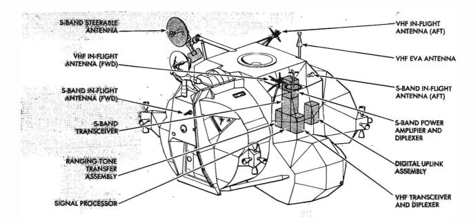
Figure 3-8.3. Communications Subsystem - Equipment Location
