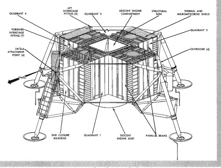
Figure 2-6. Descent Stage Structure Configuration
