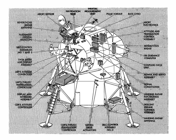
Figure 3-2.3. Guidance, Navigation, and Control Subsystem-Major Equipment Location
