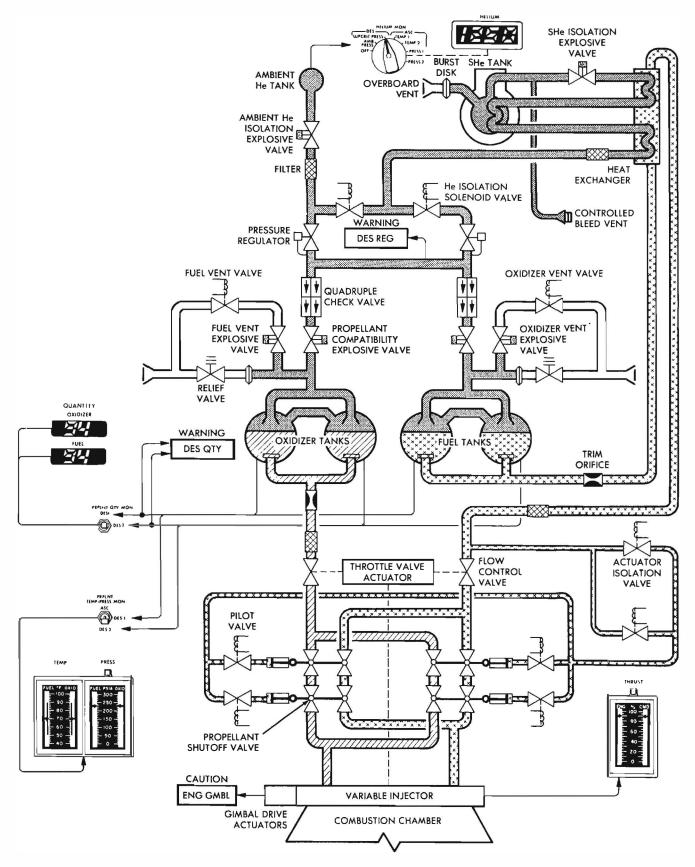
Figure 3-4.2. Descent Propulsion Section - Flow Diagram
