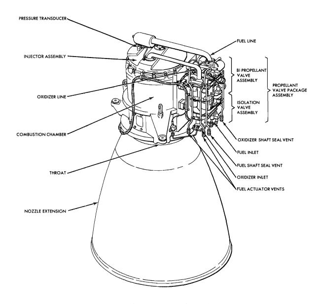
Figure 3-4.7. Ascent Engine Assembly
