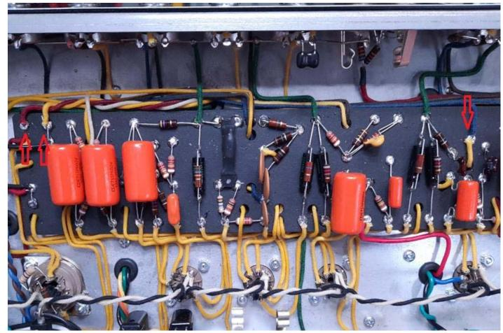
Now, set your multimeter to its highest DC reading and apply the black lead to ground (the metal chassis). Affix this in place since you will need to use your hands for holding the safety pen and the red voltmeter probe. Then ground the end of the safety pen to the ground as well.
