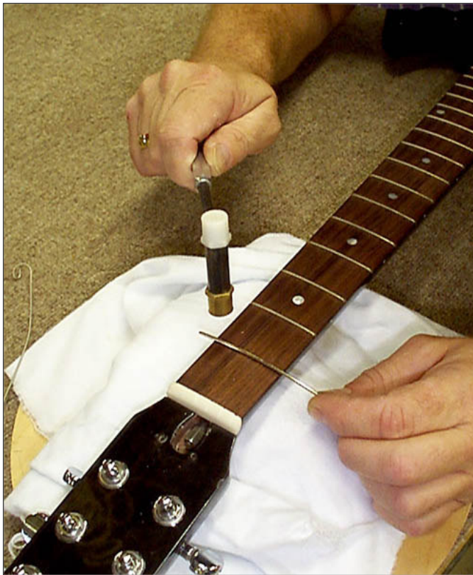
9. With flush cut pliers, trim the ends of the frets flush with fretboard.
