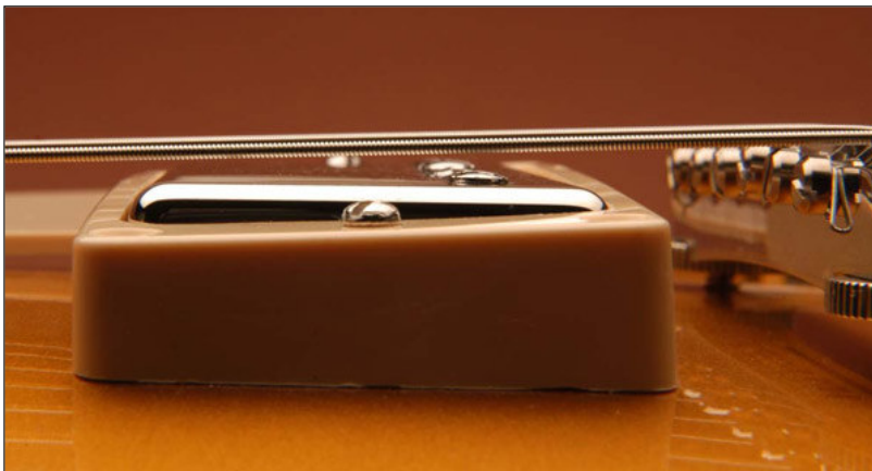
6. The Bridge: A bridge that needs to be adjusted too low or too high may be an indication of a neck that needs resetting. An improperly set neck can cause the entire guitar to play out of tune. The bridge or saddles should be intonated with a properly calibrated strobe or electronic tuner.
