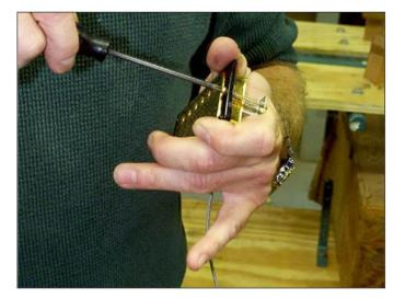
7. Snake the wire of the new pickup through to the control cavity. Then screw the pickup down to the top with the four philips-head screws, again making sure you use your free hand to old the screwdriver tip.
