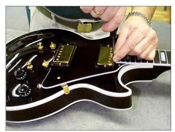
6. Mount the new pickup in the mounting ring. The spring-loaded screws can be tricky. Make sure the pickup is turned in the right direction. The neck pickup (rhythm) should have the row of polepieces close to the neck; the bridge pickup (treble) should have the polepieces on the side closest to the bridge.
