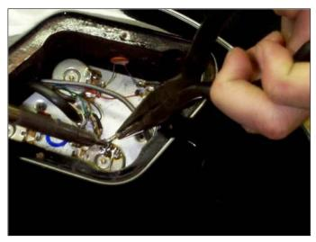
5. Remove mounting ring. Unscrew the two slot-head screws, holding your hand around the springs so that they don't pop away from you.
