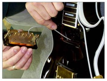
8. Solder the wires to the pot. Your pickup will either have two leads with a braided cable or (if it's wired for coil splitting) four leads.
