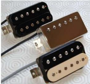
If I build a humbucker with 7,000 turns per side and coil taps 2,000 turns from each side, I get both.
