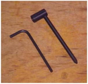
Pictured above are the two most common style of truss rod adjustment tools an Allen Wrench on the left and a barrel style socket wrench on the right, If your adjusting the neck on say an older style Strat neck you may need to use a flat bladed screwdriver instead.
