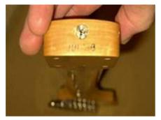
For some guitars you will find the truss rod adjustment on the other end of the neck which may mean you will have to remove the strings and take the neck off to make an adjustment.
