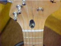
View of a standard Allen wrench style adjustment truss rod
